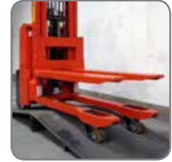
High free height makes it easy to cross edges and operate on uneven floors.
