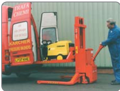
The platform being used carrying a high pressure cleaner.
