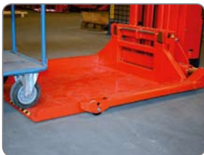
The sloping edge ensures an easy entrance to the platform.
