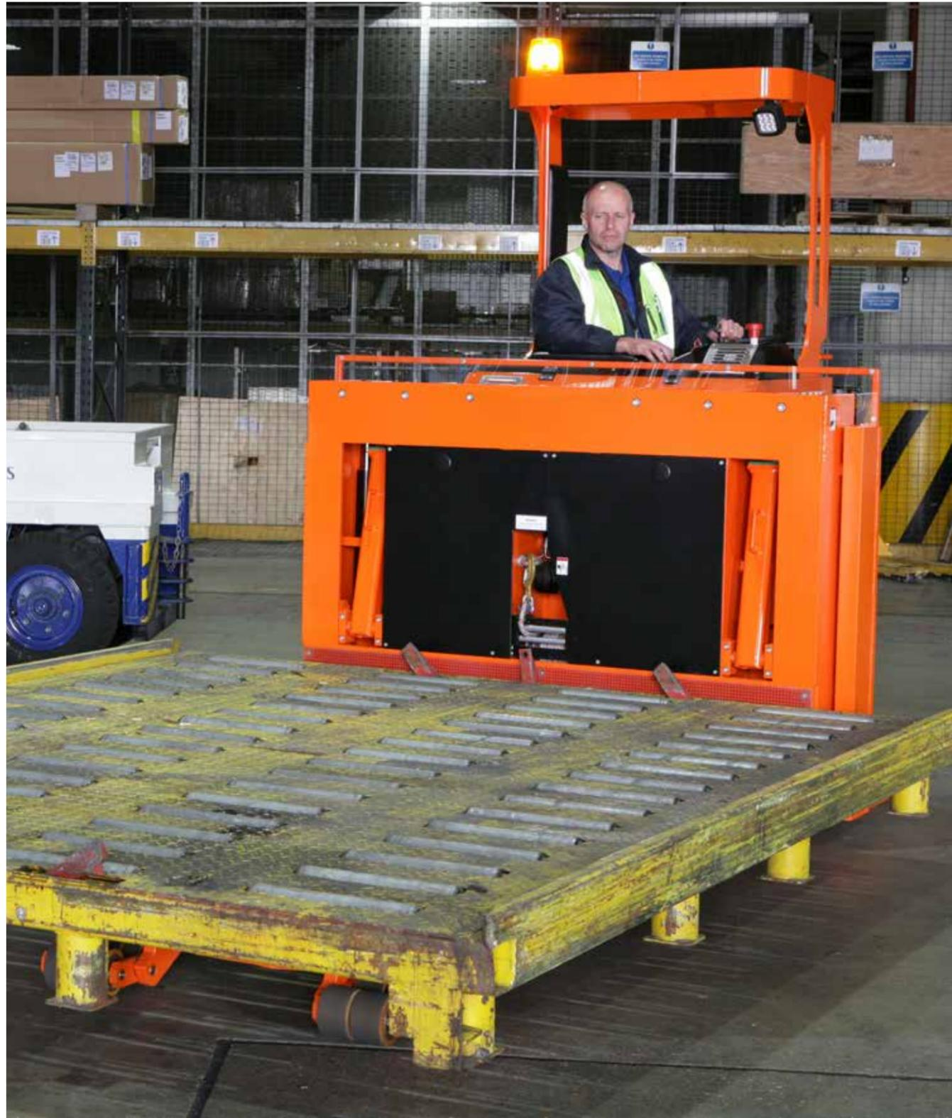
The DONKEY transports ULD's on all common slave pallet types safely and quickly and covers the whole range of the indoor transport of air cargo pallets.
