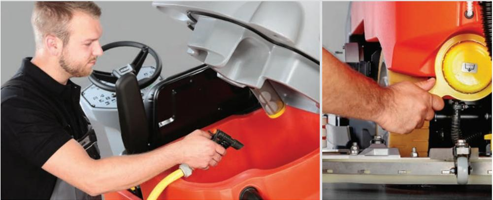
Smooth inner surfaces in the tank: makes cleaning the tank easier and prevents residual dirt from sticking to the surface. Clearly marked: All components that require regular inspection and maintenance are marked yellow.
