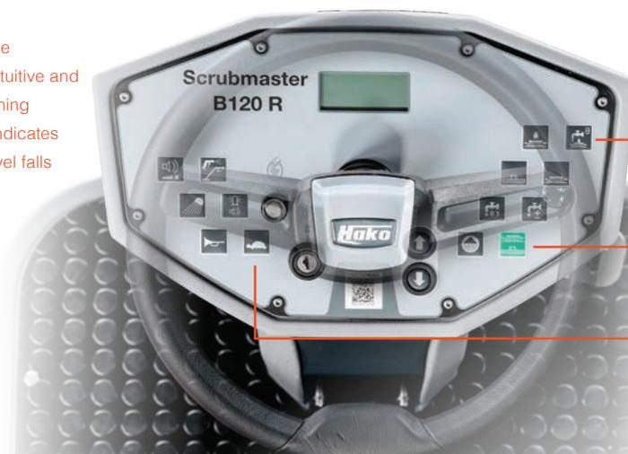
The boost button activates both maximum brush pressure and water flow.
