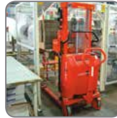
High manoeuvrability: Short overall length, large turning angle, assisted steering and low own weight.
