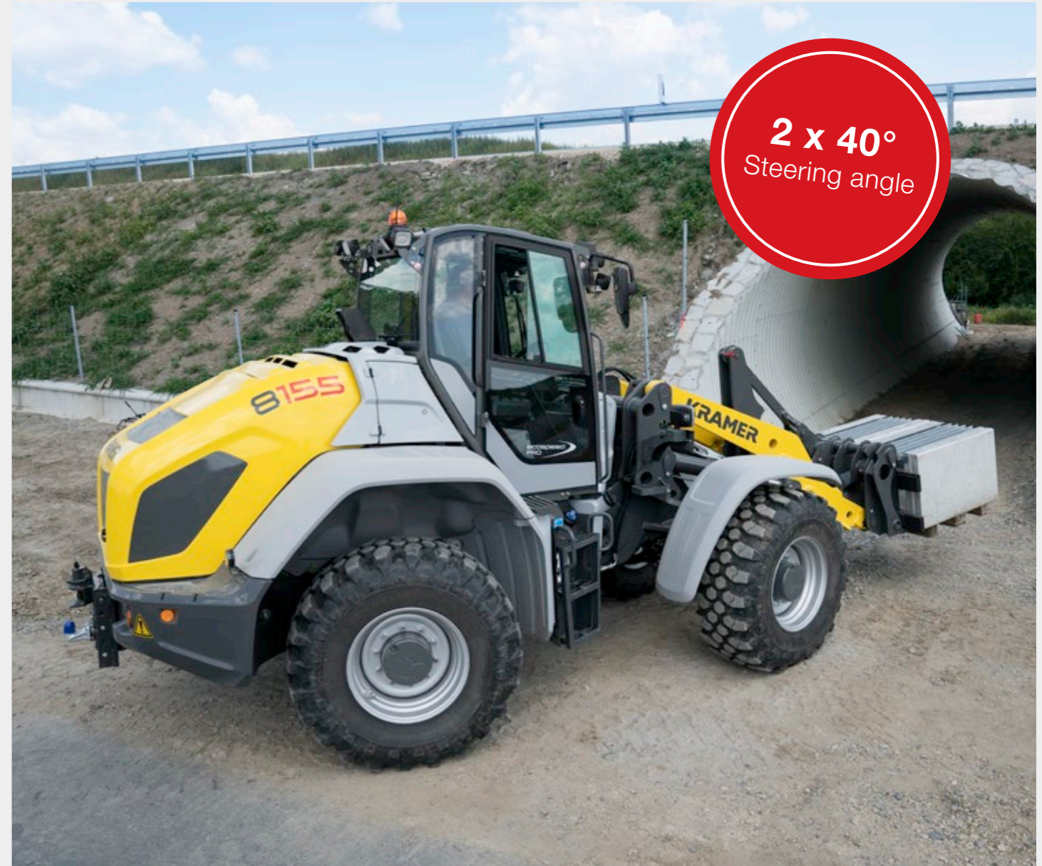
All-wheel steering particularly manoeuvrable in restricted space
