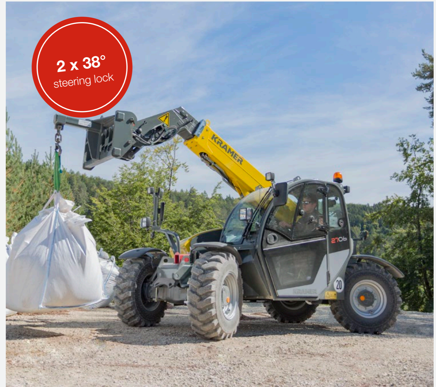
All-wheel steering: particularly manoeuvrable in tight spaces
