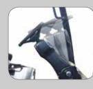
**Fully Adjustible Operator Compartment** The steering column, as well as the full suspension comfort seat, armrest and optional headrest, are all adjustable to accommodate individual preferences for each forklift operator.
