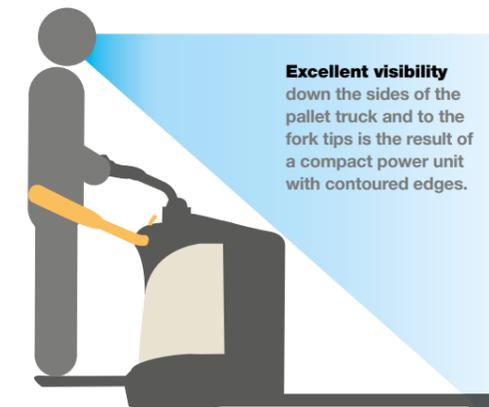
Excellent visibility down the sides of the pallet truck and to the fork tips is the result of a compact power unit with contoured edges.
