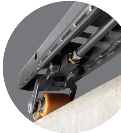
**One-piece high tensile steel forks** are formed into a C-channel and reinforced in critical areas. An adjustable pull-rod lift linkage eliminates buckling forces and elevates the riser axle for protection.
