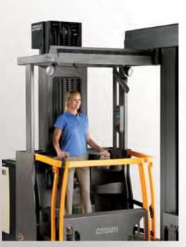
Tasks that benefit from standing are efficiently accomplished with a seat that folds up and controls that adjust to the ideal operator height.
