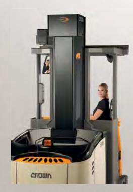
The sloped power unit design and flexible seat positions give the operator a clear view of the aisle improving manoeuvrability and operation in and out
