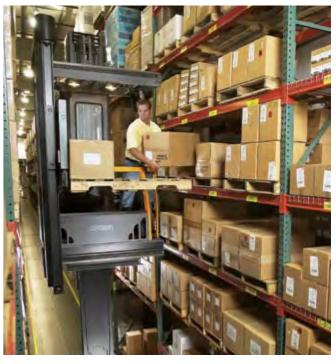
**ORDER PICKING:** Sturdy steel side gates and clear front rail reduce the need for operators to bend or lean when retrieving product from the rack or placing it on a pallet. In addition, the rails can be used to support the weight of the product as it is transferred.
