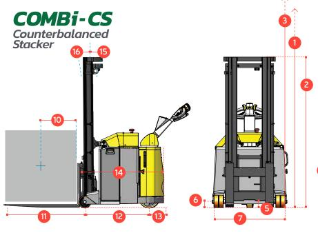
With a load capacity of 1000kg @ 500mm the Combi-Counterbalanced Stacker (Combi-CS)can work in the smallest operating aisles.
