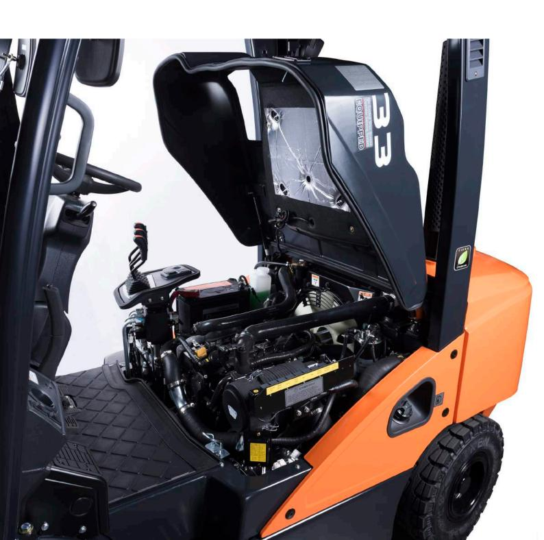
All our powerful diesel and LPG engines are compliant to the current regulations for reduced emissions. These in-line, 4-cylinder, water cooled, overhead valve engines provide high torque at low engine speeds for applications requiring ramp loading and unloading, fast lift speeds, or heavy hydraulic flow requirements.
