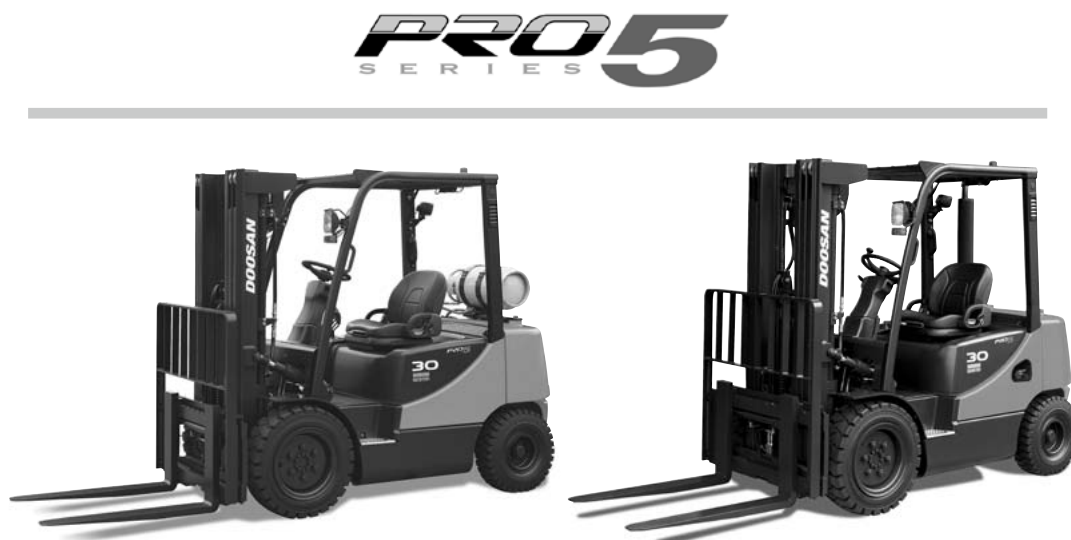
G20E / G25E / G30E-5 G20P / G25P / G30P / G33P-5 & G35C-5 2,000kg 2,500kg 3,000kg 3,300kg 3,500kg LP, Pneumatic Tire
